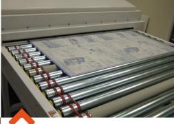
Optional infeed and exit (cooling) roller conveyors.
