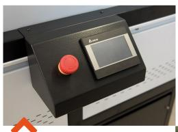
Full colour LCD Touchscreen HMI Display provides access to all control functions and displays all plate baking parameters.
