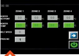
Individual control over the four baking zones and belt speeds.
