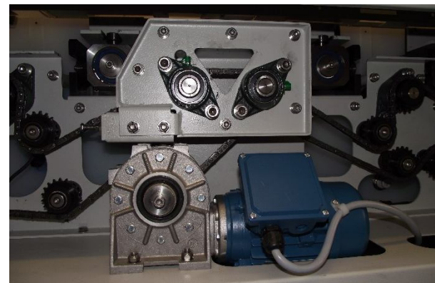
TWP 1250 - Heavy duty chain drive system with AC drive and brush motors. Idlers fitted with sealed ball race bearings for maintenance free operation
