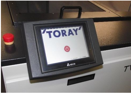
Full Colour LCD Touch Screen HMI Display provides access to all control functions and displays all processing parameters
