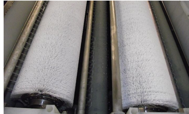
Large diameter rotating and oscillating brush rollers ensure optimum removal of softened silicone layer and application of after-treatment (dye) solution
